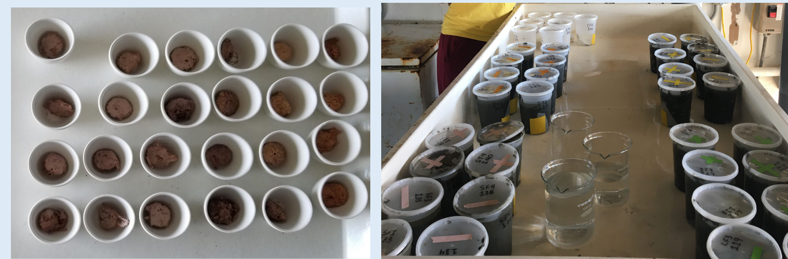
Figure 2: Sediments being prepped for Loss-on-ignition (Organic Matter Content) (left) and the mesocosms (right)
