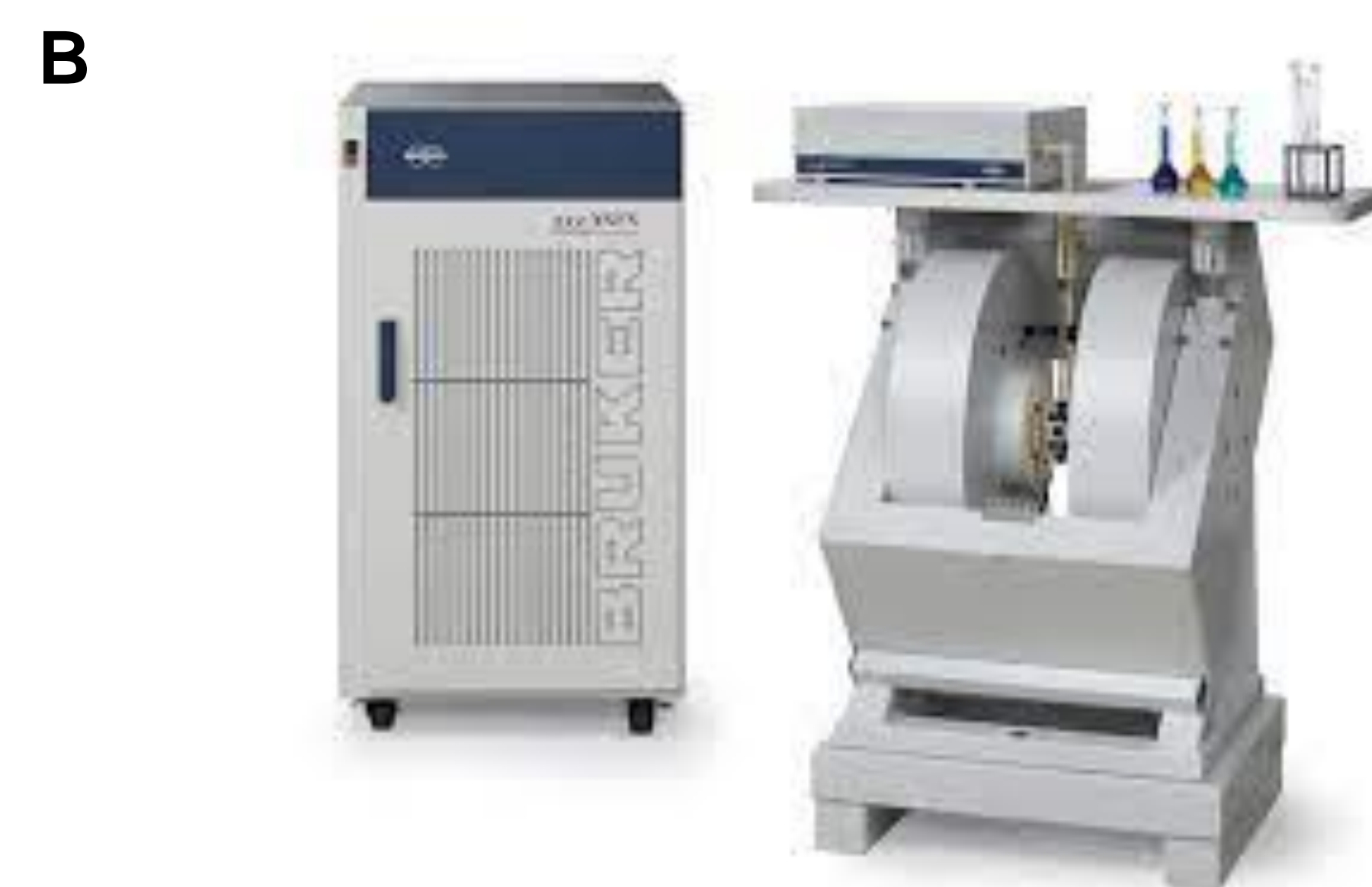
Figure 4. (A) EPR spectra of Gd:WO_{3-x} samples on an X-Band ELEXSYS EPR Spectrometer (B) Image of BRUKER ELEXSYS EPR Spectrometer
