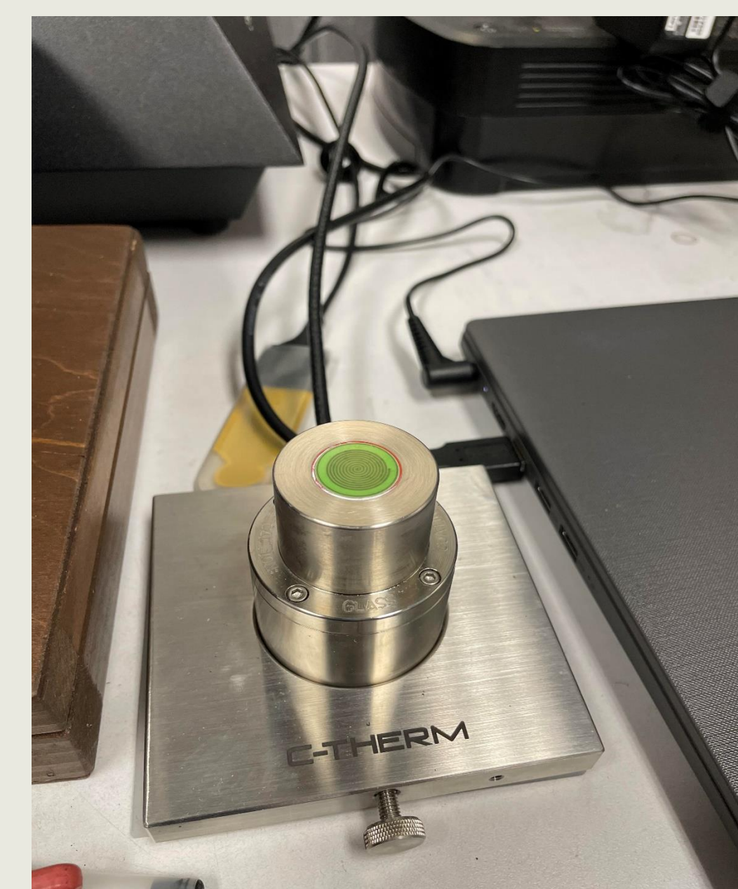
Above: C-Therm trident sensor used to measure samples thermal conductivity
