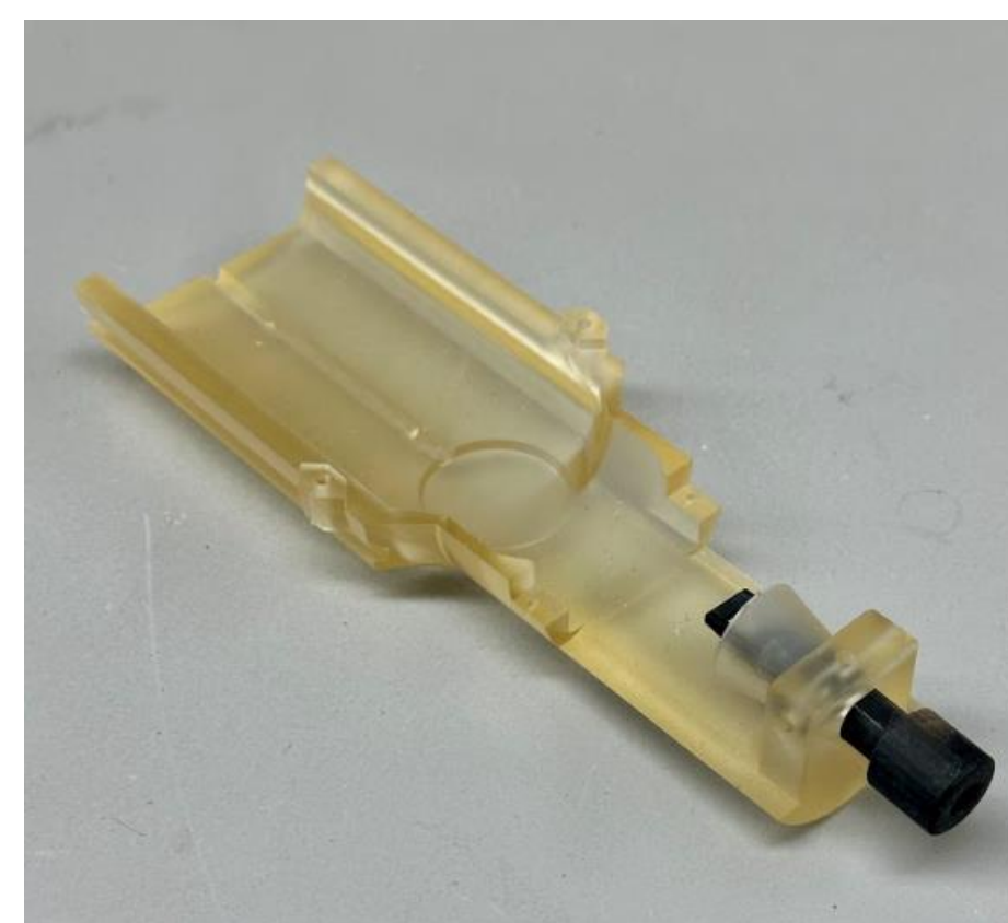
Figure 2: Stereotaxic rodent cradle used in preclinical MRI studies [2]
