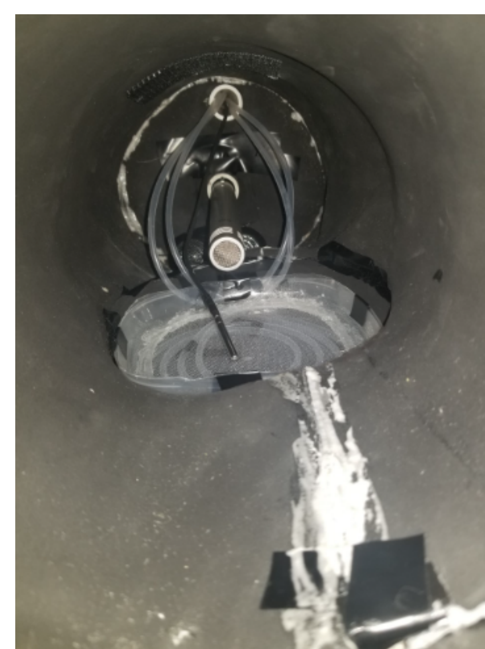
Fig. 1 Inside of a recording chamber, containing a round speaker to play chorus sounds to the male being recorded. Chorus frogs do not usually call in silence, so chorus sounds are necessary to stimulate calling.
