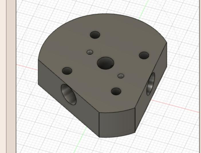
To the right, the attachment by which a mirror will reflect phosphorescence into a quartz rod. On the left, the sample holder itself.
