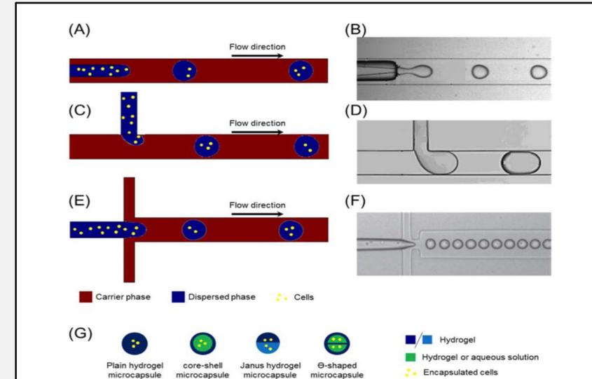
Figure 6. Image by Huang *et al.* in *Generation and Manipulation of Hydrogel Microcapsules by Droplet-Based Microfluidics on Mammalian Cell Culture* shows the three different basic microfluidic devices that are used for cell encapsulation with a variation in the schematics of the generation system.
