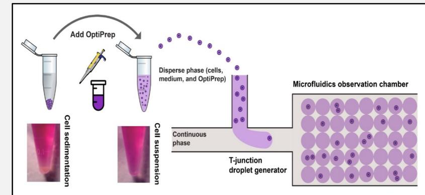
Figure 5. Image by Liu *et al.* in *Improving Single Cell Efficiency and Reliability through Neutral Buoyancy of Suspension* shows single-cell encapsulation process with human monocytic OptiPrep™ to create a neutral buoyancy of suspension.
