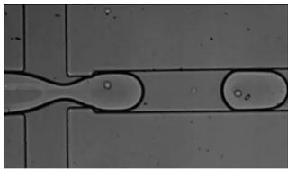
Figure 1. Image from *Microfluidic Droplet Production Method* by Fluigent, captures high droplet generation frequency and the low volume of the microfluidic system.
