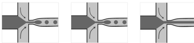
Figure 2. Image reference from *Microfluidic Droplet Production Method* by Fluigent, captures varying regime formation of droplet generation system, ranging dripping, jetting, and stable co-flow regime.
