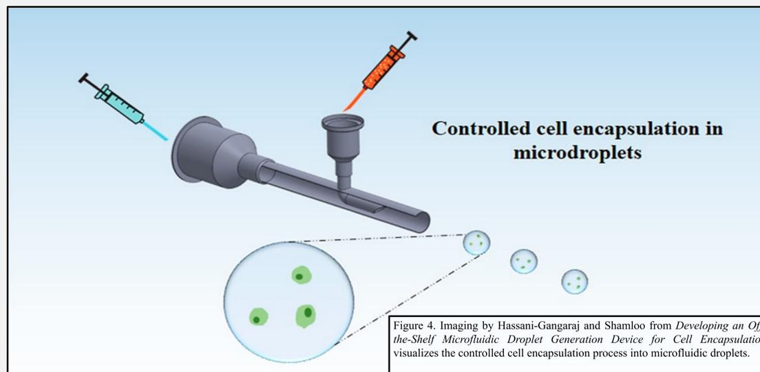
Figure 4. Imaging by Hassani-Gangaraj and Shamloo from *Developing an Off-the-Shelf Microfluidic Droplet Generation Device for Cell Encapsulation* visualizes the controlled cell encapsulation process into microfluidic droplets.
