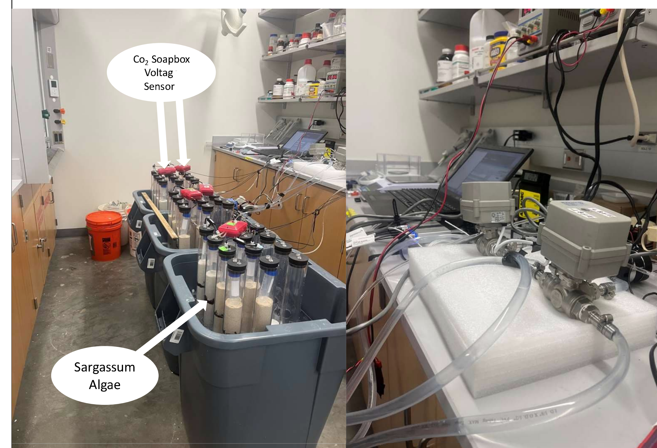
Tidal pumping containers with algae packed sediment columns (Left). Pump timing mechanism used to switch tides (Right)
