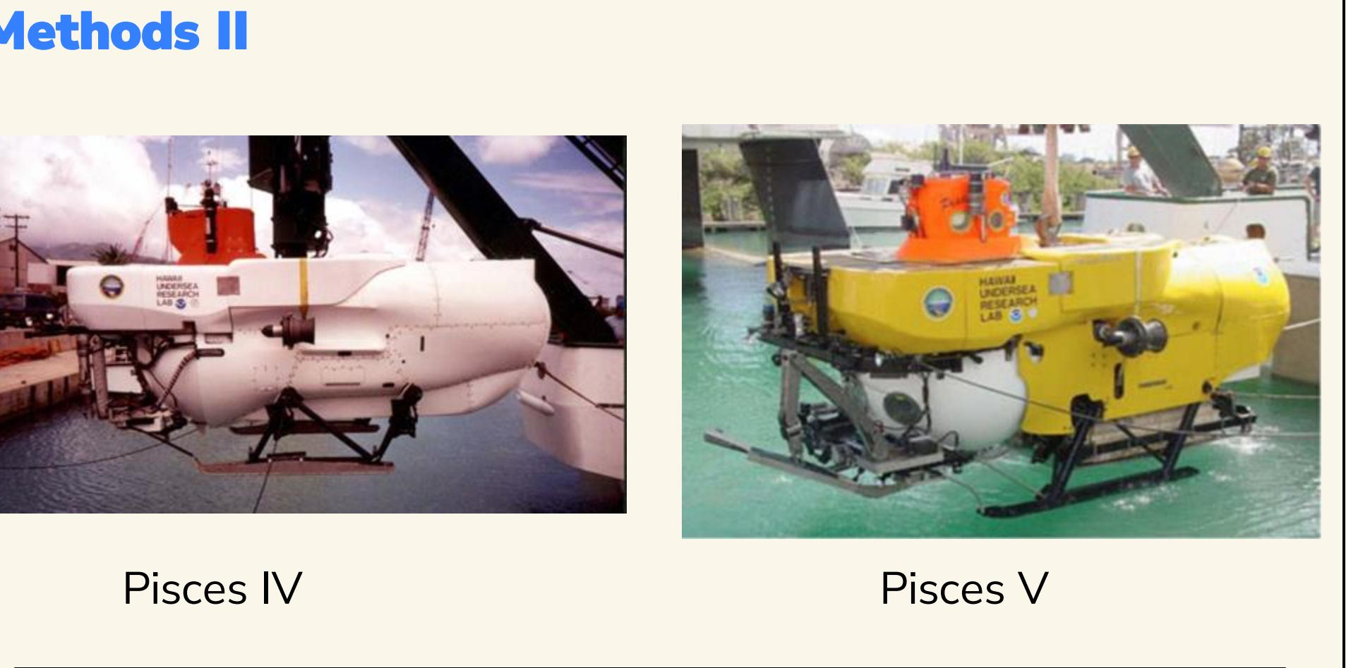
**Figure 1 and 2. Images of the human-occupied deep-submergence vehicles used to collect video footage of the seamounts.**
