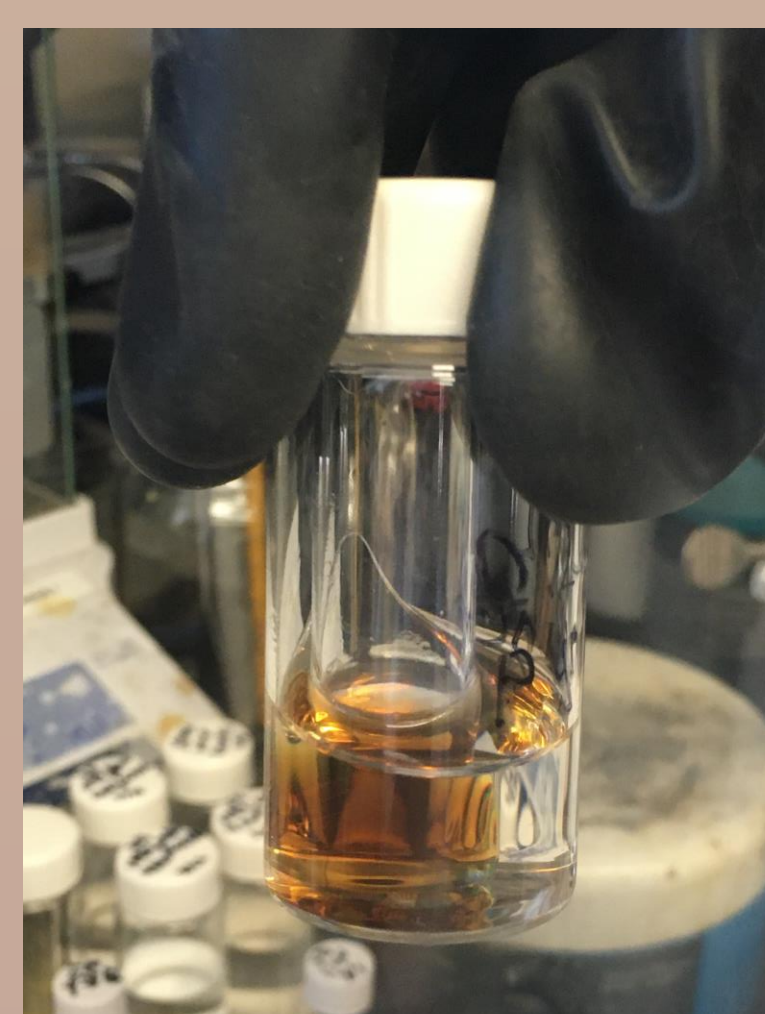
18C BDT, EuI 3 , and pyridine solution in pentane vapor diffusion
