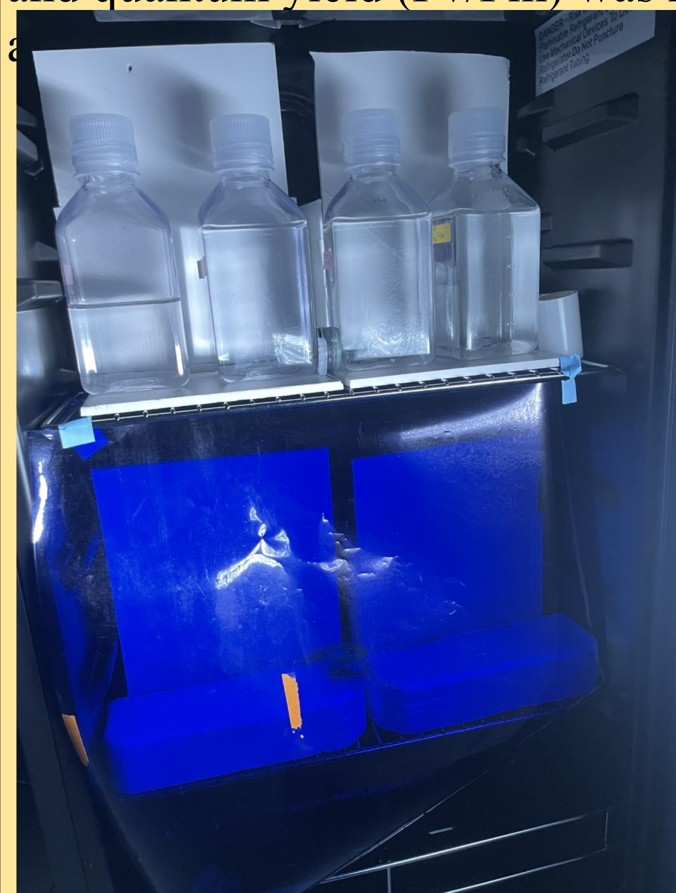
Figure 3: Constant incubation setup for Thalassiosira Antarctica . Top row = high light adapted bottles. Bottom row = low light adapted bottles. Light was supplied by a LED light array.
