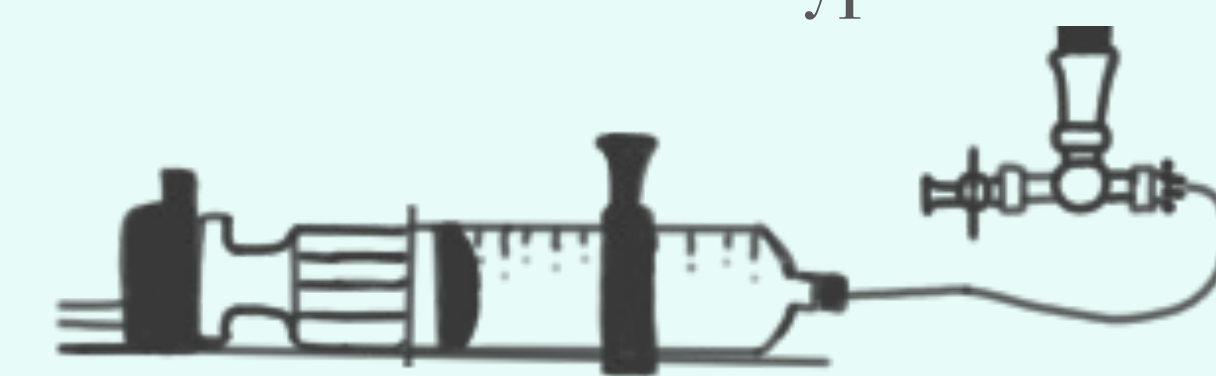
Fig. 3b. The connection of the water-filled syringe (which is emptied by the infusion pump) to the bottom of the column.
