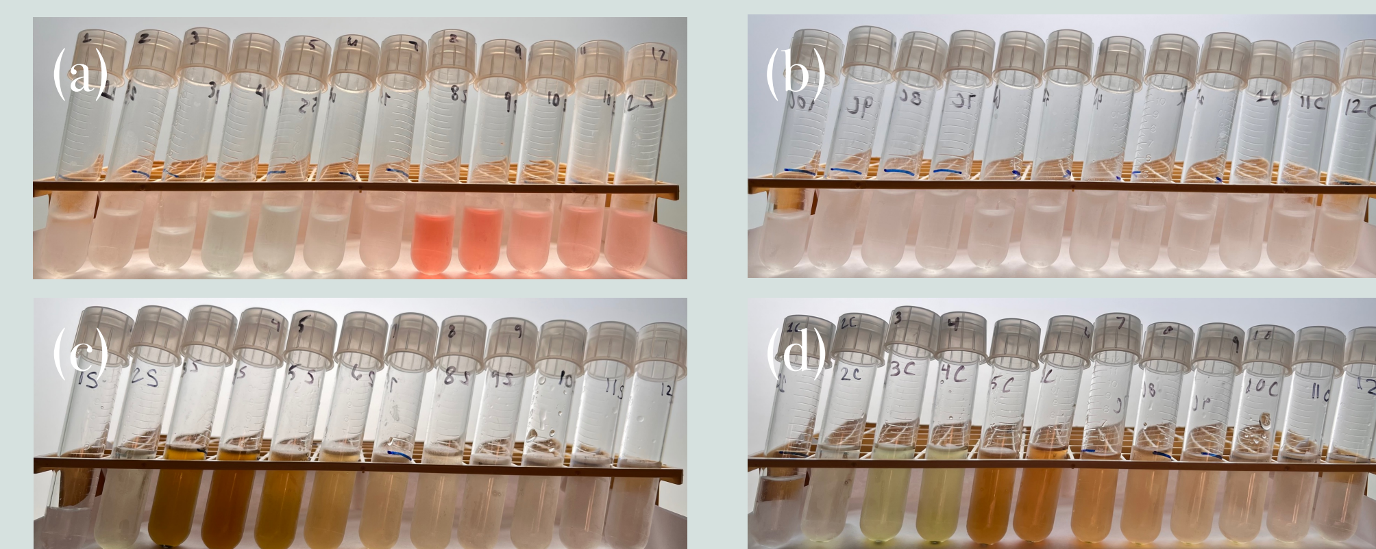
Fig 4. Samples collected when running organic dye through (a) \text{SiO}_2 and (b) \text{CO}_3 sands; and phytoplankton pigments through (c) \text{SiO}_2 and (d) \text{CO}_3 sands; shows the color separation over time in the two sediments.
