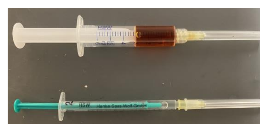
Figure IV: Top: 3 mL Sulfur/OLAM Injection Bottom: 1 mL DDT Injection
