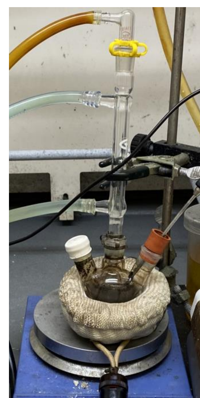
Figure I: Round-Bottom Flask Reactor Middle Neck: Condenser Right Neck: Thermocouple
