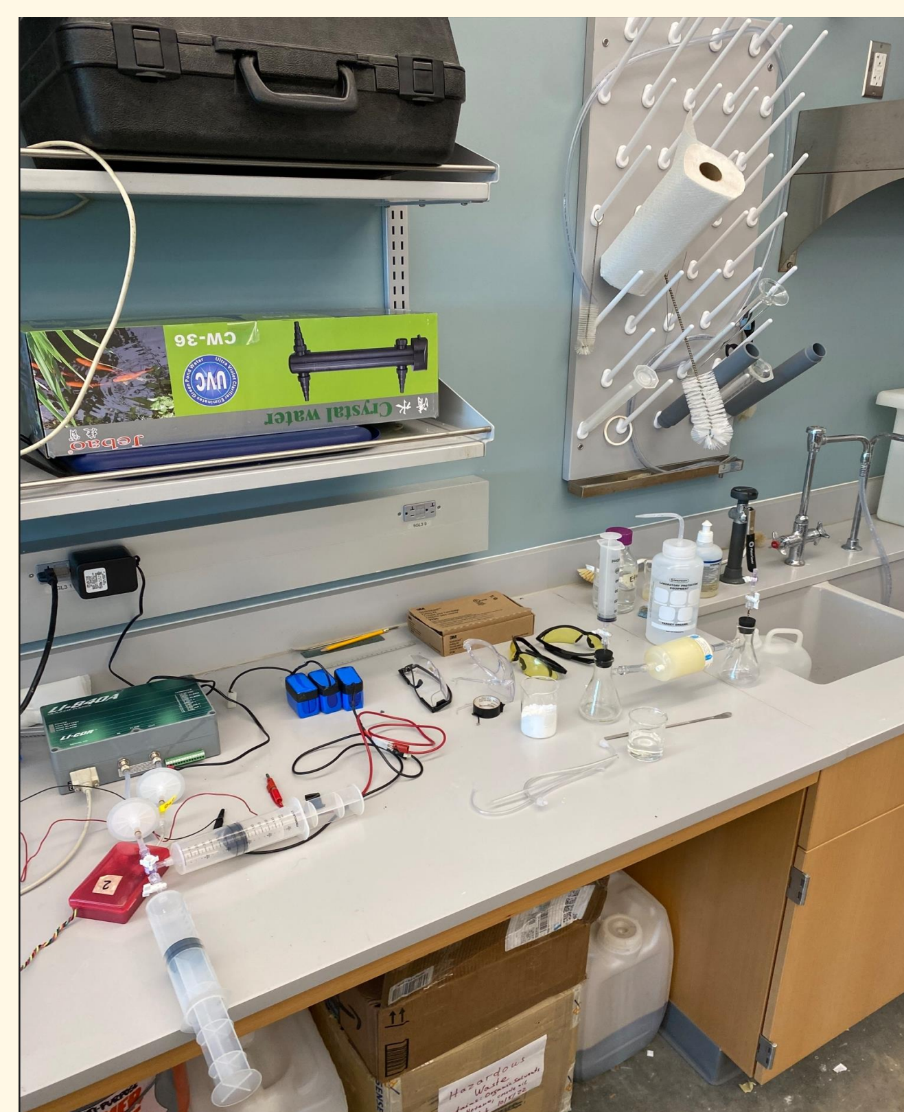
Figure 3. Calibration of Pyroscience Oxygen Optode, LiCor LI-850A CO 2 Sensor, and custom-made CO 2 sensor.
