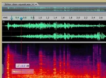
Instead of studying amplitude over time, the CNN studies the spectrographs of audio as frequency over time so that it can be compared and classified.
