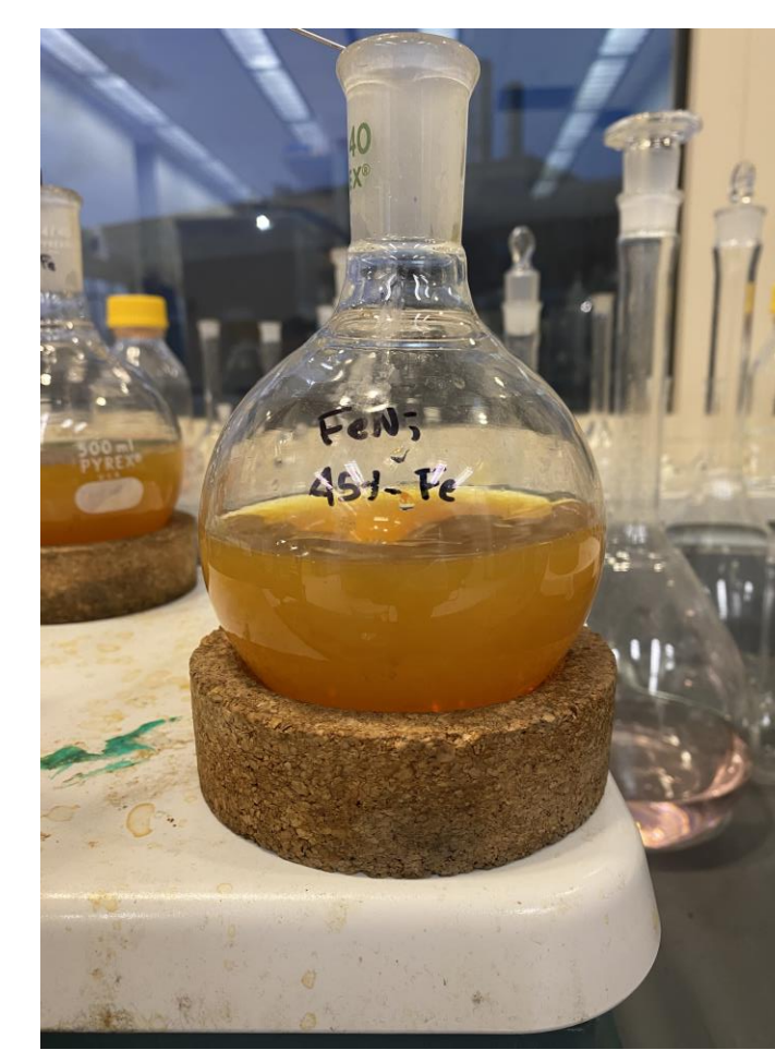
FeNi PBA synthesis at a ratio of 45% Fe.
