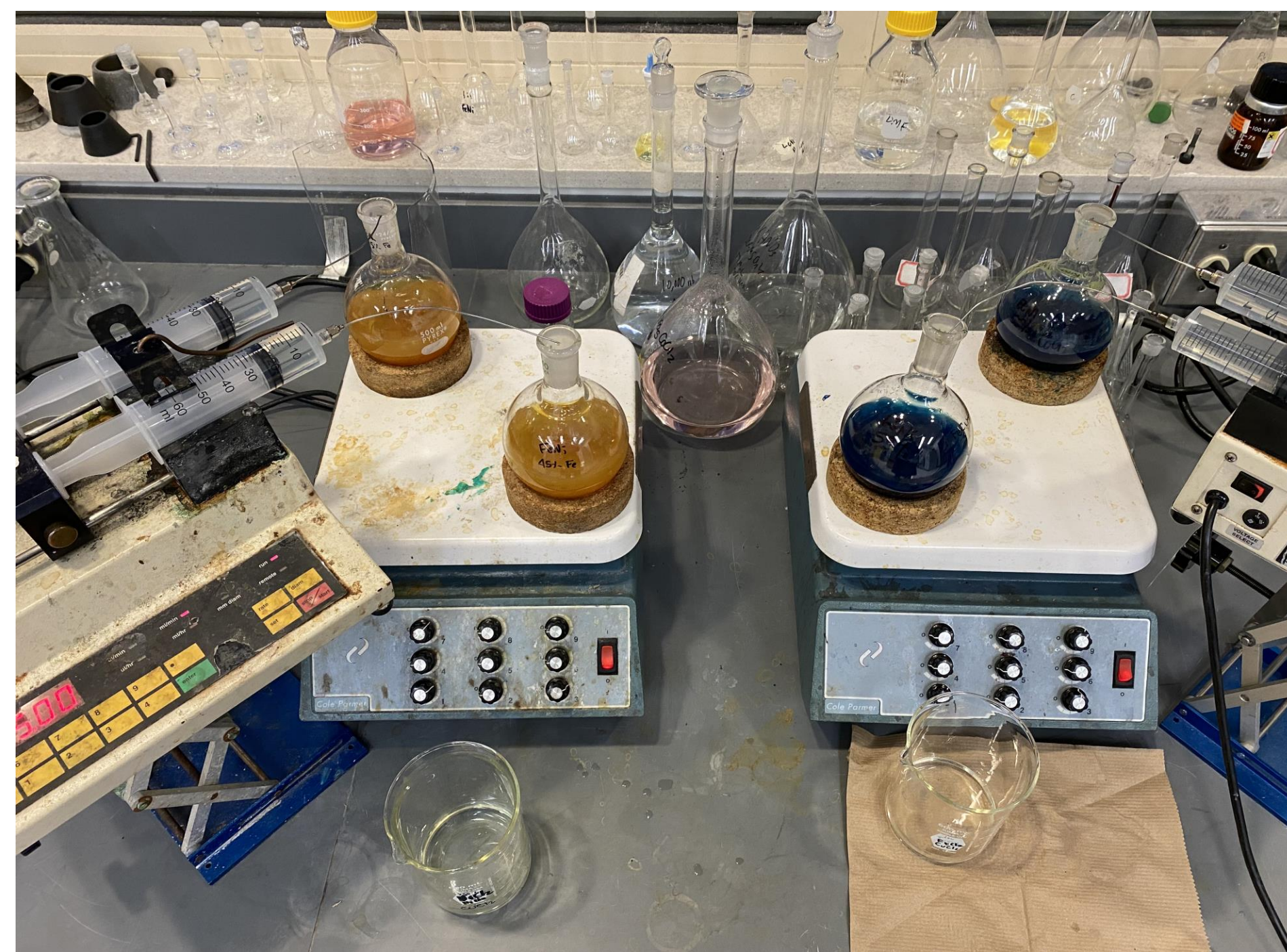
FeNi PBA synthesis at different ratios. NiCl 2 is added via syringe to the two samples on the left, and FeCl 2 to the two samples on the right.
