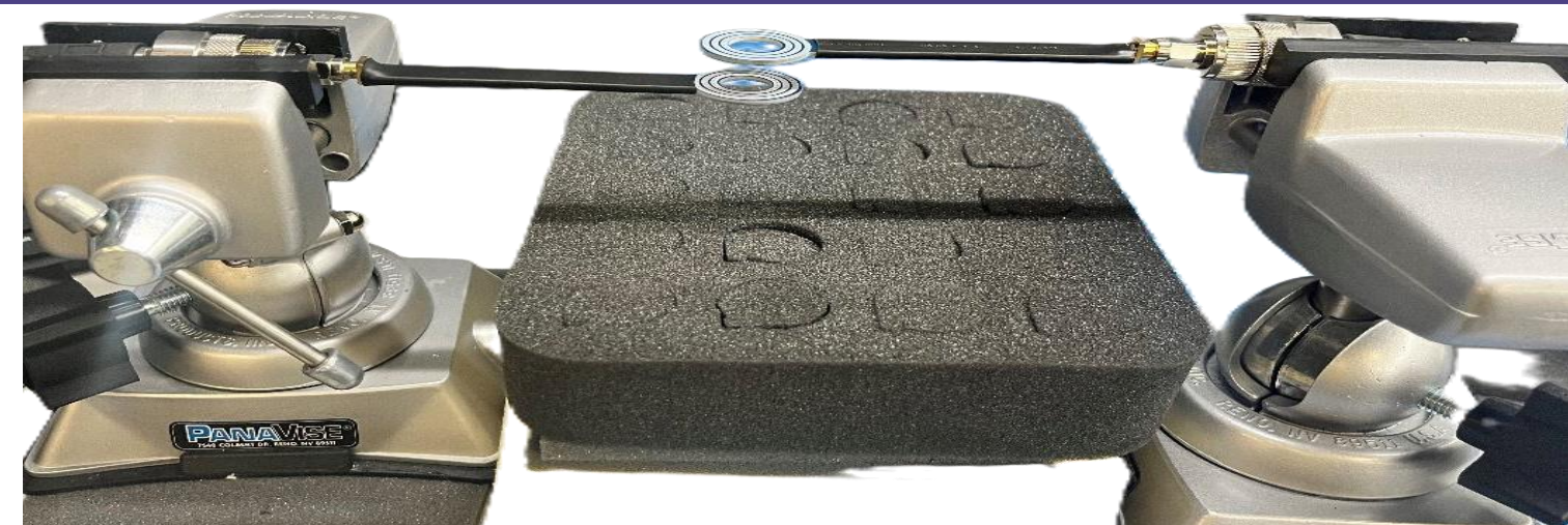
FIGURE 3: VNA pick-up loop configuration used for normalization
