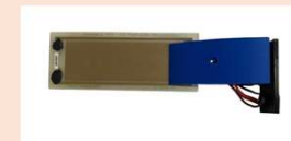
MFC Strip Used in Experiments
