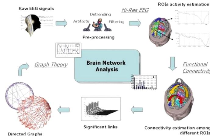
EEG processing pipeline for brain network analysis, transforming raw signals into functional connectivity graphs for seizure prediction.
