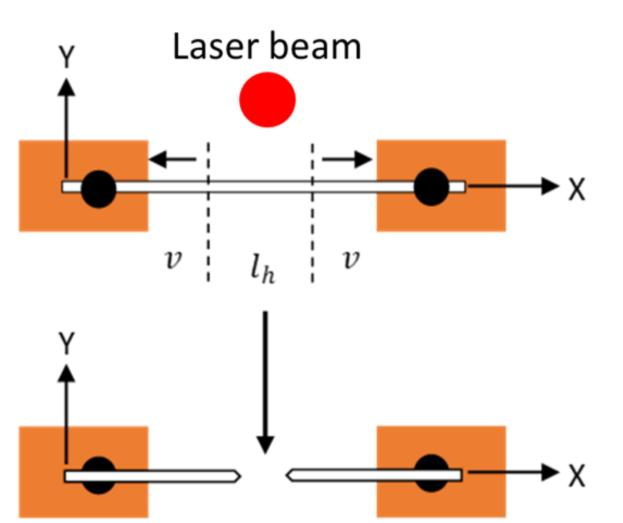
Nanopipettes are fabricated from quartz
