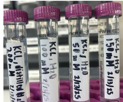
Figure 1: KCl Samples: 50mM, 100mM, 150mM, 200mM
