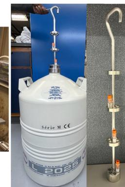
Figure 2e: Cryogenic Dipper in liquid nitrogen tank
