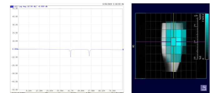
Figure 3a: Tuning of 39K coil @41.7 MHz
