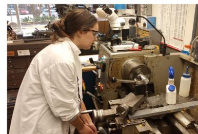
Figure 2d: Lathe used to machine a diameter of 1.85" on each plate
