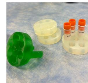
Figure 2c: 3D Printed Cryovial Plates
