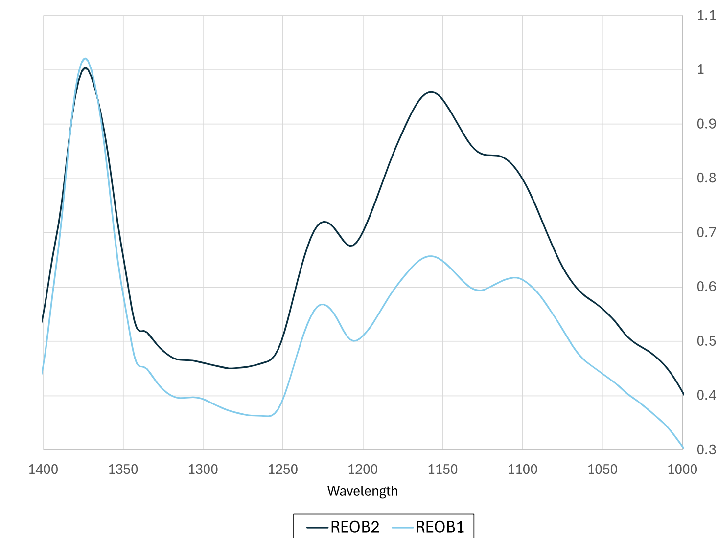
Fig. 6: FTIR Comparison of REOBs
