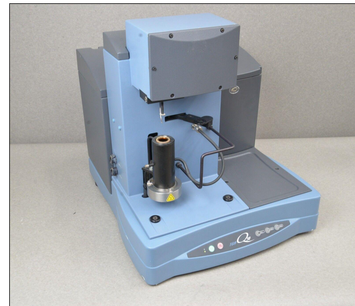
Fig. 3: Q50 Thermogravimetric analyzer
