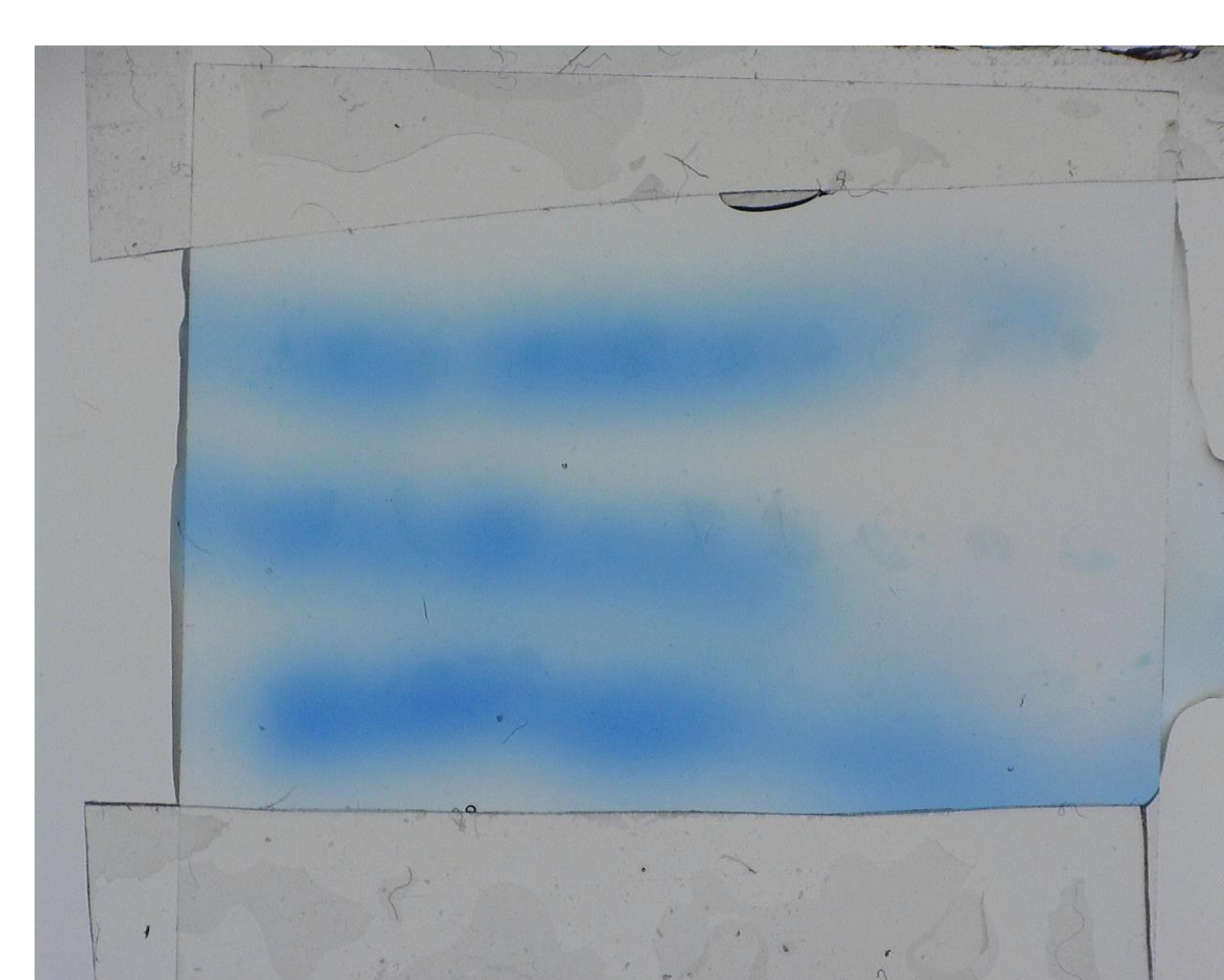
Figure 5. Droplets flowed with copper solution resulting in methylene blue dye displacement.
