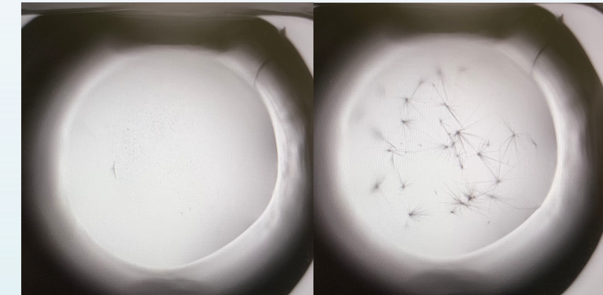
Figure 3: Both images shown below are of the same well in a crystal screening, but they are taken at different times. The image on the left shows the well taken on day 0. The image on the right was taken on day 10 and shows the beginning of crystal growth, referred to as "needles".
