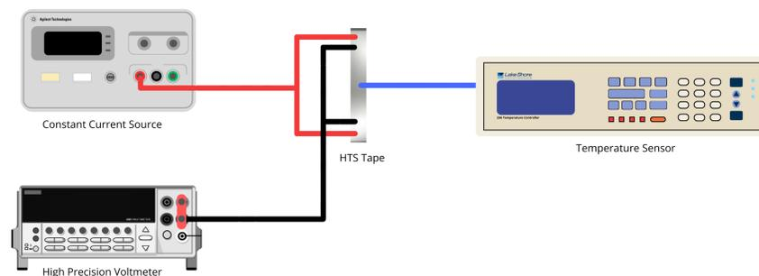
Figure 3: Experiment setup for measuring the critical temperature of HTS tape
