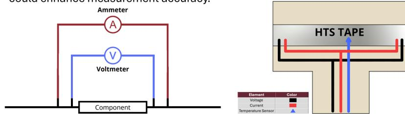
Figure 1: Four-Probe Method
