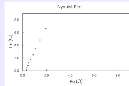
Figure 2 - Nyquist plot measured from electrochemical impedance spectroscopy of p5PhS-Na
