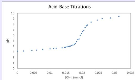
Figure 1 - Acid-Base Titrations after ionic exchange between p5PhS-Na & NaCl
