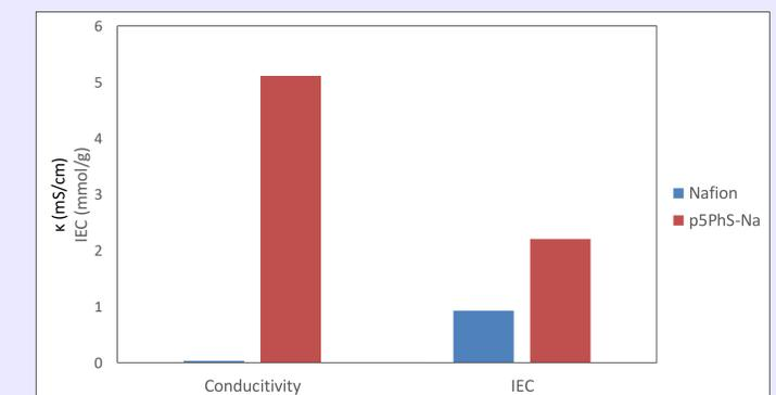
Figure 4 - Bar graph of ionic conductivity & IEC of Nafion & p5PhS-Na
