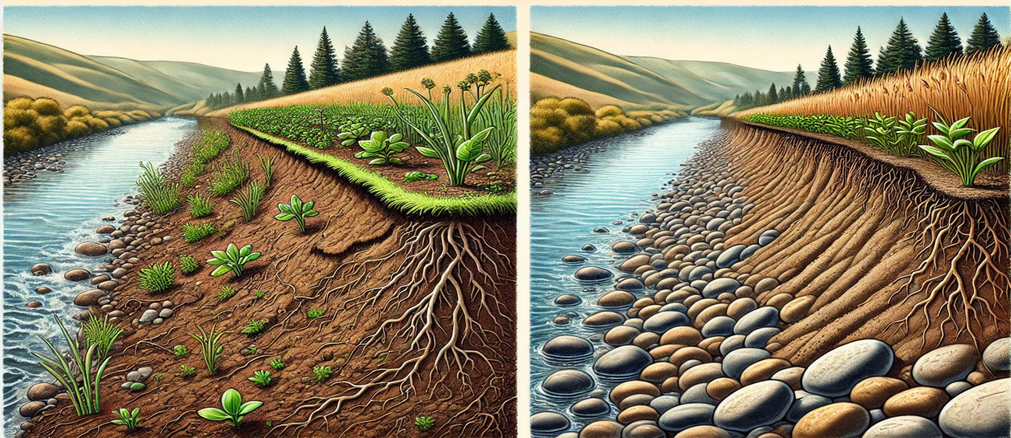
A model of vegetation seeding on the left and rock armoring on the right
