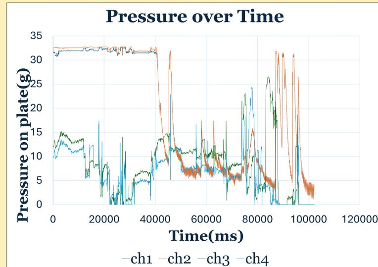
Figure 1: UA-R4-W30 bucket tested. Sensors (CH1, CH2, CH3, CH4) were attached to the top left, top right, bottom left, and bottom right corners of the plate, respectively.
