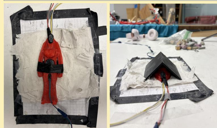
Figures 3 (Left): Picture of 3-D printed human; sensors attached to critical parts of the human body (head, chest, & stomach).
