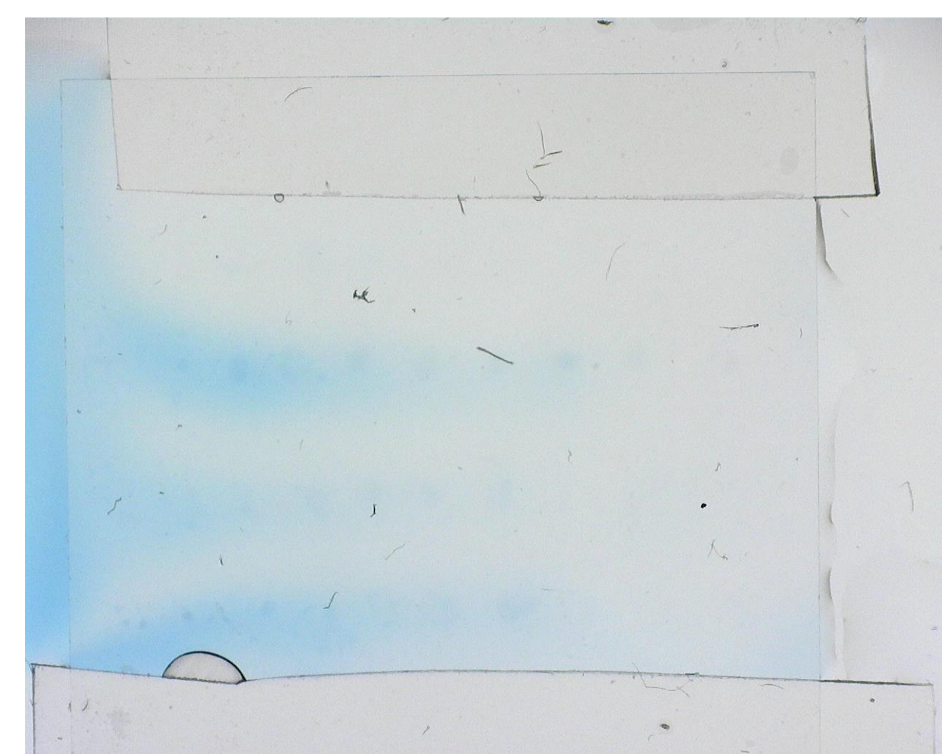
Figure 4. Droplets flowed with lead solution resulting in displacement.
