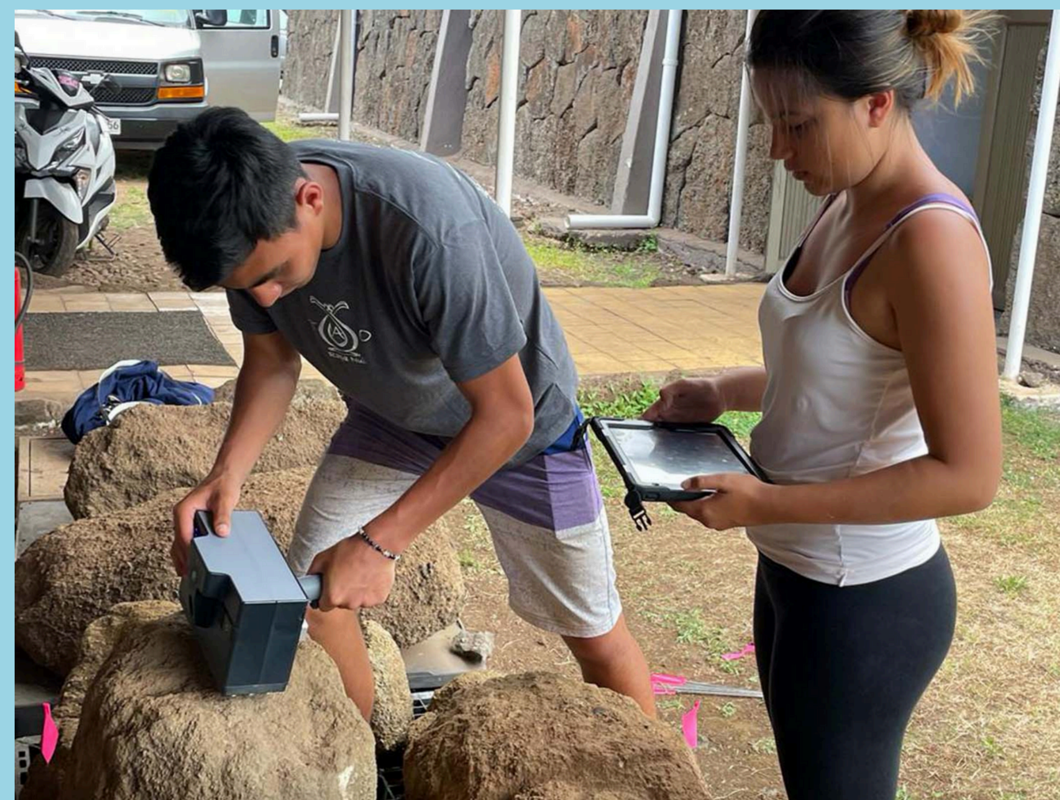
Students use an ultrasonic scanner on fragments of stone tuff, Courtesy of the TAO
