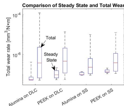
Figure 4: Steady State and Total Wear Rate Comparison
