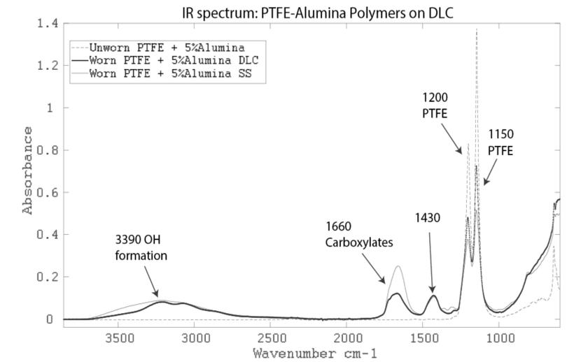
Figure 3: Alumina FTIR Comparison
