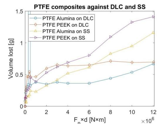
Figure 5: Volume Lost vs Normal Load times Distance
