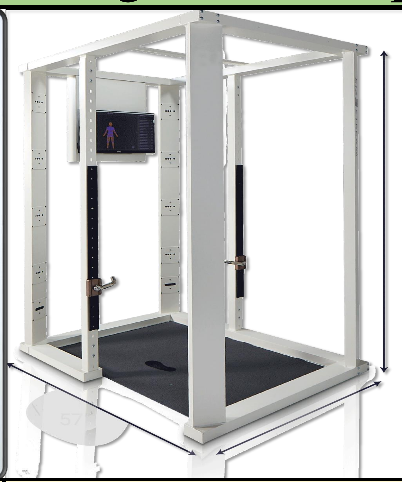
Figure 3 : SS20 Scanner used for the 3D body scans of the firefighters.
