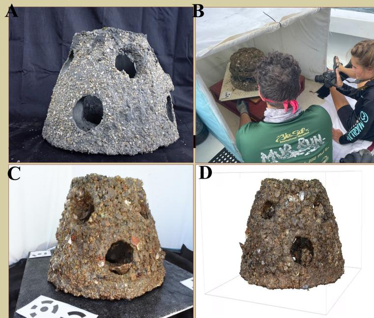
**Figure 2: Reef Ball photogrammetric development**
