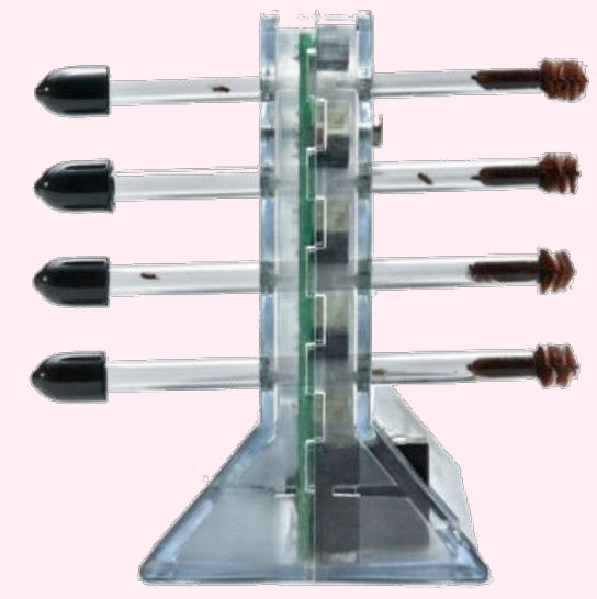
Figure 1. The Drosophila Activity Monitoring (DAM) system. Sleep was measured starting at ZT0 and averaged over 3 days (Pfeiffenberger et al. , 2010).
