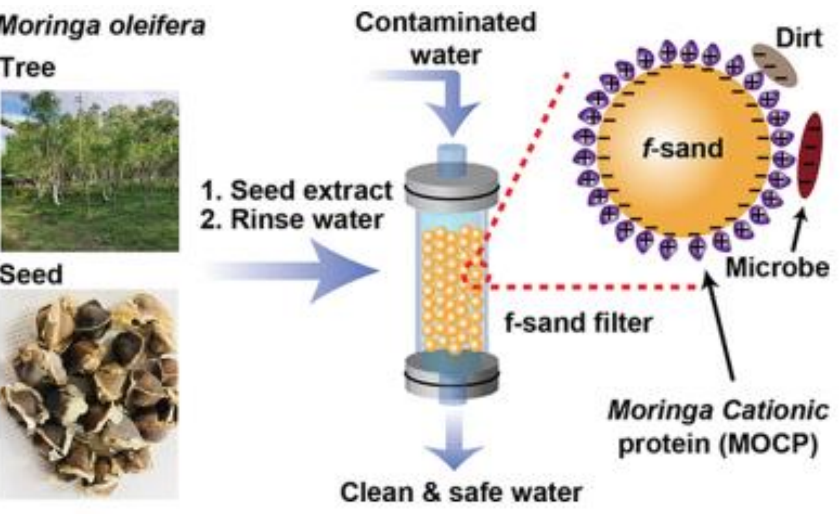
Figure 1. (Xiong et al., 2017) Shows the mechanism of action by which cationic protein coats the surface of sand particles to reverse their charge and bind to anionic particles. Moringa tree and seed are shown on the left. Column sand filter experiment from the literature shown in the middle. Sand coated with positively charged moringa serum and bound negatively charged particles on the right.
