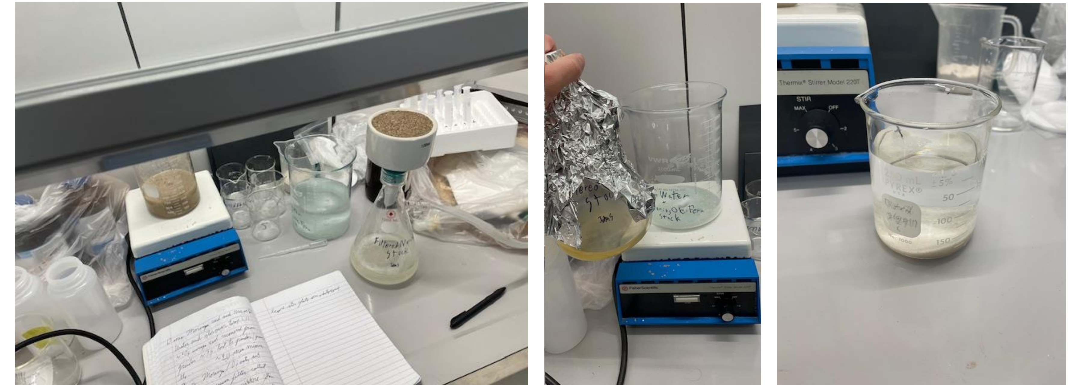
Figure 4. Shows multiple components of the F-Sand creation Procedure. Figure 5. shows Moringa oleifera extract serum and SiO2 bead substrate (sand). Figure 6. shows an early batch experiment.
