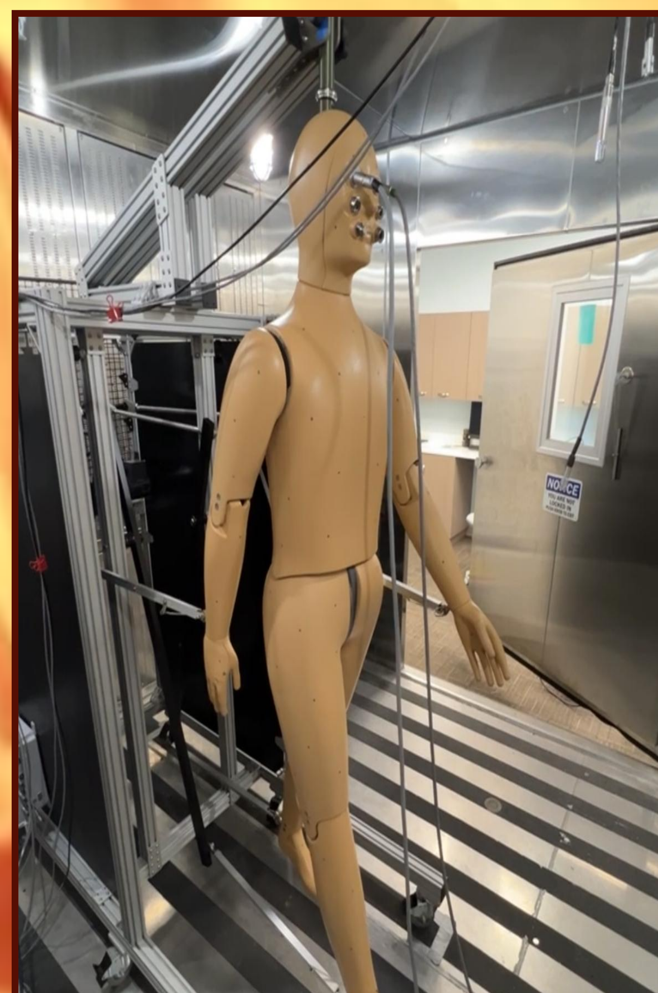
ANDI Manikin in the FSU ThermaNOLE Comfort Lab®
